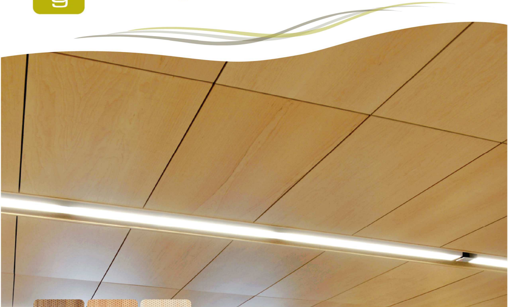
Photo: Microperf Ceiling Panels, Maple Plain Sliced Veneer, 11/16" Particle Board Core, Custom Stain, .5mm Perforation, Soundtex applied to back, Lift & Twist Mounting
